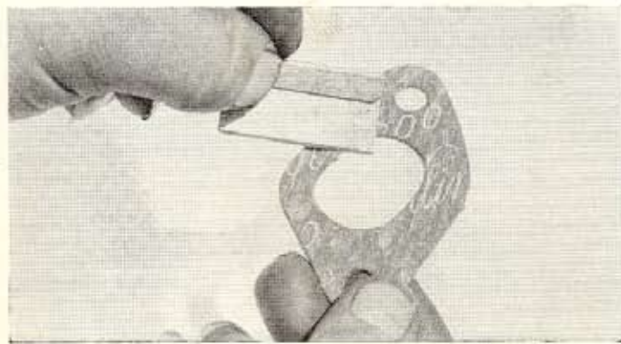
Induction manifold gasket is cut back to stop it squeezing and obstructing port when it's bolted up.
