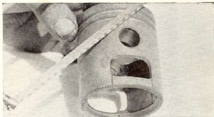
The 'window' in the piston is cut out more to lessen drag and also to advance the port timings.
