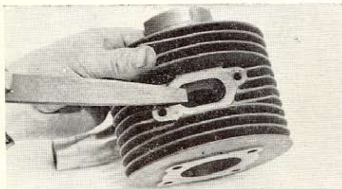
Gas flow through the inlet and exhaust ports can be helped by filing away smooth any rough edges.
