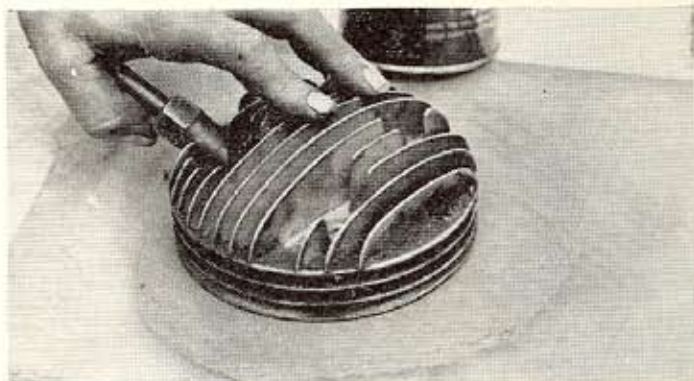
To skim down cylinder head, use an old mirror or piece of plate glass and fine carborundum paste.
