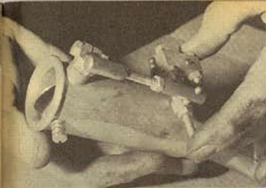
An alternative to the Amal concentric carb in the inlet department is this Wal Phillips fuel injector. Specially made for both Lambretta and Vespa models, it costs about £8. And is well worth it!
