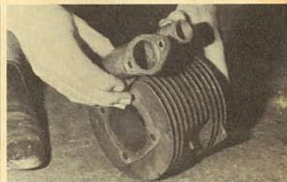
If you're using a big carburettor or fuel injector then you will need an inlet manifold to match it. The one on the left is 1 1/2 in. Just compare it with the standard manifold on the right
