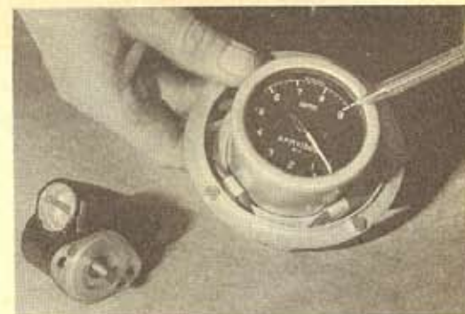
If your bike has been tuned to any extent you will need a rev-counter. Then you will be able to calculate performance gains as well as being able to avoid damaging the engine by over-revving it
