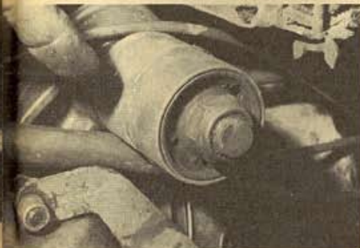
The double engine mount, of bonded rubber in a steel ring, makes a vast improvement to the handling. Stops twitching when accelerating from a bend. A really necessary fitting for fast scooterists
