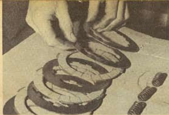
The Lambretta clutch shows a tendency to slip if constant high revs are used on take-off. To eliminate this an extra steel plate is used to pack out the assembly. No problems if this mod is done
