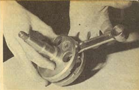
A special long-stroke con-rod assembly that Supertune have developed to give the Lambretta a capacity of 247 cc! At present it is just experimental but may be in production soon. Should be fantastic
