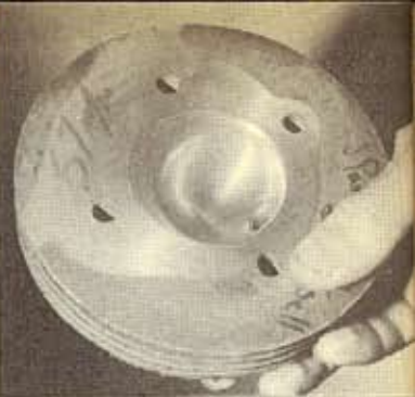
Cylinder head skimming is standard practice in two-stroke tuning; this one, from a Lambretta 150 has had 0.060 in. taken off. Radius edge of combustion space to clear piston
