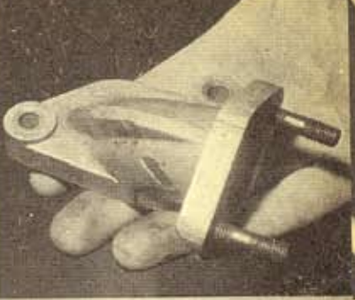
Although the inlet port doesn't need altering, performance benefits from this inlet manifold which will accept either an Amal Monobloc or a Wal Phillips "injector"
