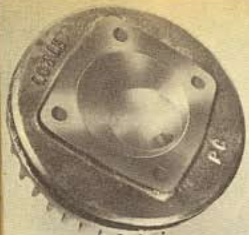
An alternative for Lambretta owners is to buy one of these 10:1 c.r. heads made by George Todd. They cost £4 16s. 6d. each, and that includes the correct NGK sports spark plug
