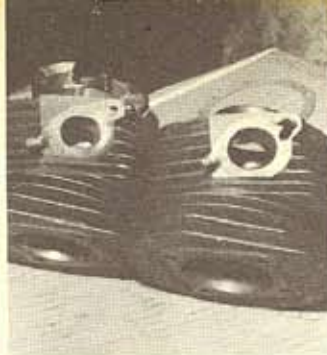
Wildcat's bore out to increase capacity and on a full race job they will also open out the inlet and exhaust ports. Compare with standard hole left
