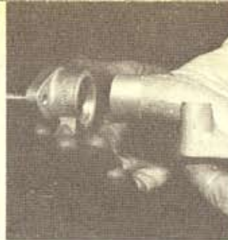
. . . flange-fitting Amal is adapted to stub by use of Wildcat adapter. Manifold and adapter must be filed if necessary to match the size of carb
