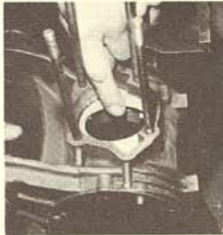
This primary compression plate (or crankcase stuffer) drops into barrel hole and is nipped lightly by the barrel. It increases crankcase compression
