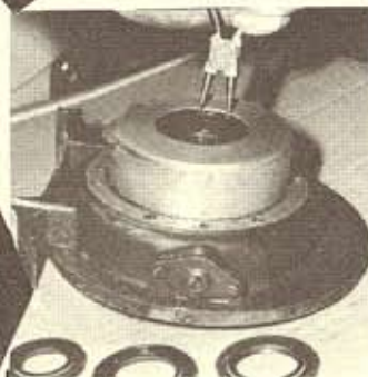
Always replace the three crankshaft seals whenever you take the crank out. They are held by circlips, with main bearing between seals on timing side
