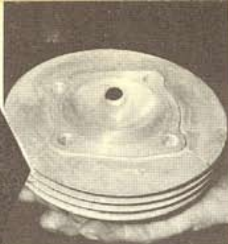
This is the side-squish head used on everything except the 125 GP. You can't do much about improving it, so the best thing is a 125 GP head, or...
