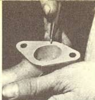
Many inlet manifolds are available, and the main thing is to open the bore to match the modded barrel and an Amal Concentric carb. The . . .
