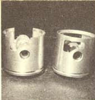
. . . you have a converted barrel, you can also cut the bottoms off the transfer port windows, as per the Dykes piston on the left. The \frac{1}{16} is still removed
