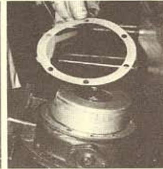
Next step in the battle for case compression is to leave out the gasket 'twixt the faces. This can be safely done on all models Use smear of gasket goo instead
