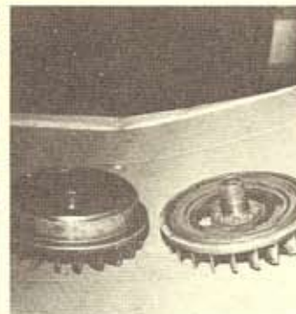
. . . while on later jobs. If you don't mind having no charging system, the flywheel can be lightened thus: you will have to use separate coil . . .
