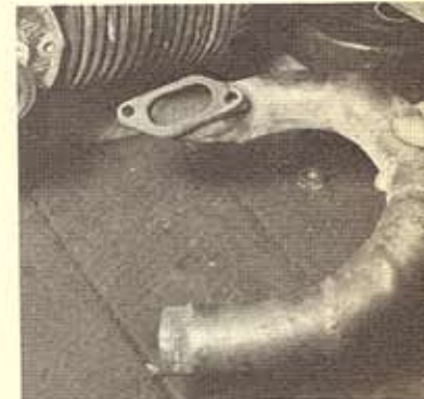
There is no special exhaust pipe available, but one can easily be made up for use with silencer — see below
