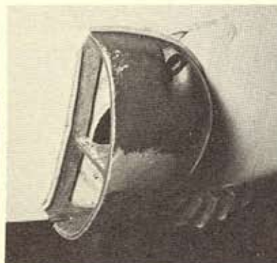
A larger carb may require a cutaway in the cover—this kind of air scoop can easily be made up and fitted
