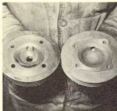
Cylinder heads can be machined down to give higher compression ratio. Central plug may be fitted to central squish-type head
