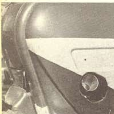
Another way of improving your breathing on a tuned motor! Cut a hole in the side panel, jet up the carb, and fit a bellmouth
