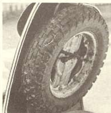
For improved traction on sprint hill climbs this Continental studded tyre was fitted. It is also handy as a spare for road
