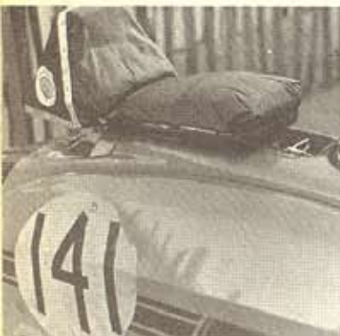
Another home-made device to get the rider down behind the handlebars. It may not be comfortable, but leaves filler free
