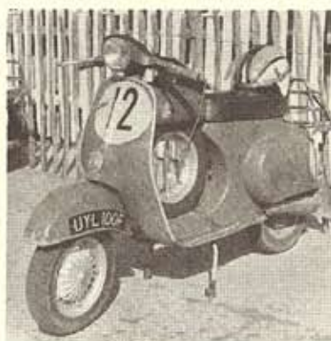
Virtually standard apart from the tank-top padding with score/navigation board, this Vespa Super Sprint won a "master" award
