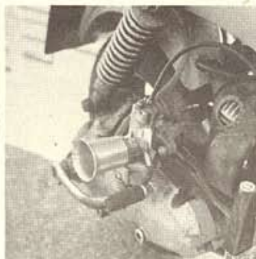
A 125 cc conversion is now possible on the Luna and to obtain better breathing this Amal concentric carb is fitted as shown
